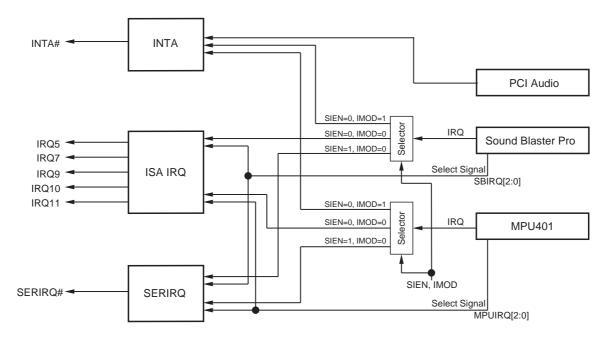
PCI Audio can only use INTA#, but the Sound Blaster Pro and MPU401 blocks of the Legacy Audio Block can use any of the three protocols.
