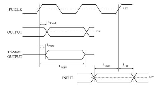
Fig.4: PCI Bus Signals timing
