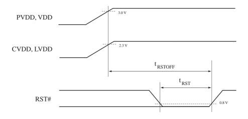
Fig.2: PCI Reset timing
