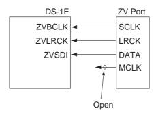
The Zoomed Video Port is used to be selected between SPDIF input on YMF744B (DS-1S). However, on DS-1E, the both functions can be used at the same time.
