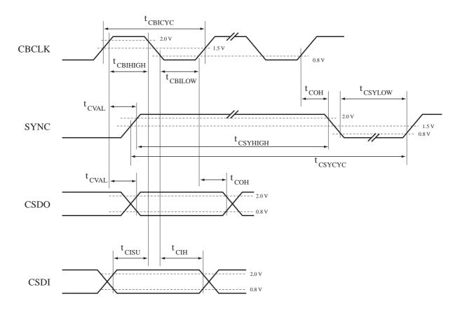
Fig.6: AC-link timing
