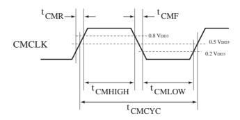
Fig.5: Master Clock timing for AC'97
