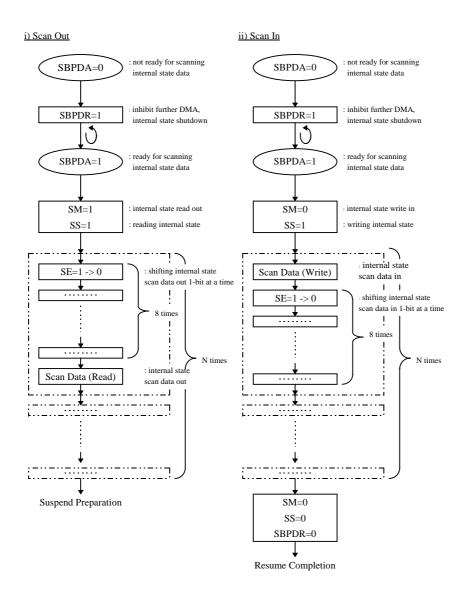
N = 34 byte (Total Scan Data = 268 bit (33 byte x 8 + 4 bit))
