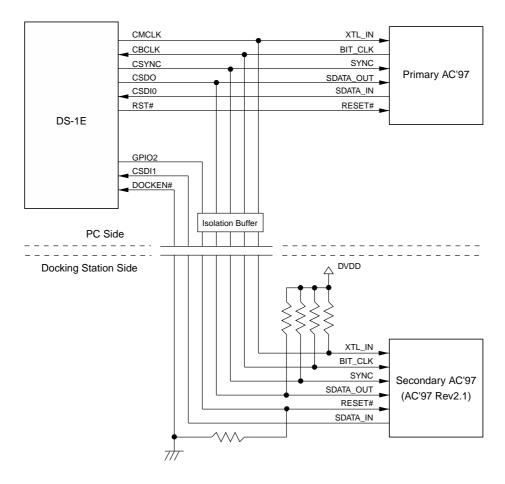
When digital docking interface is made with the main side (PC side) powered on, but docking station side powered off, it may be not desirable for the secondary AC'97 that each output signal from the AC-Link is applied to the secondary AC'97 that remains in powered off state. In order to avoid such a situation, it is necessary to place an additional isolation buffer on the PC side (or docking station side).
