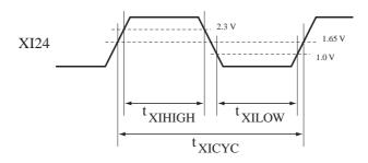
Fig.1: XI24 Master Clock timing
