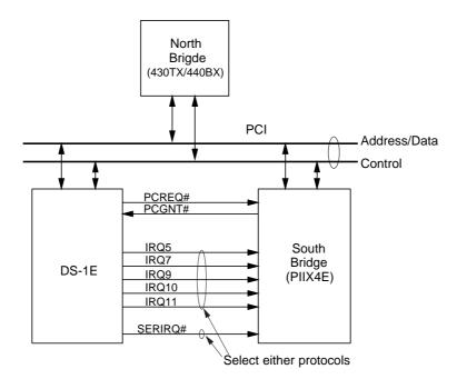
The PCI-to-ISA bridge needs to support PC/PCI. IRQ is directly connected to the IRQ input pins on the PCI-to-ISA bridge.
