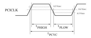
Fig.3: PCI Clock timing
