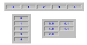
Figure 32. QHBoxLayout, QVBoxLayout, and QGridLayout
