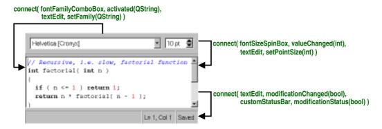
Figure 11. An example of signals and slots connections
