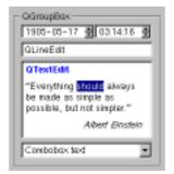
Figure 5. A QDateTimeEdit, a QLineEdit, a QTextEdit, and a QComboBox laid out with a QGroupBox
