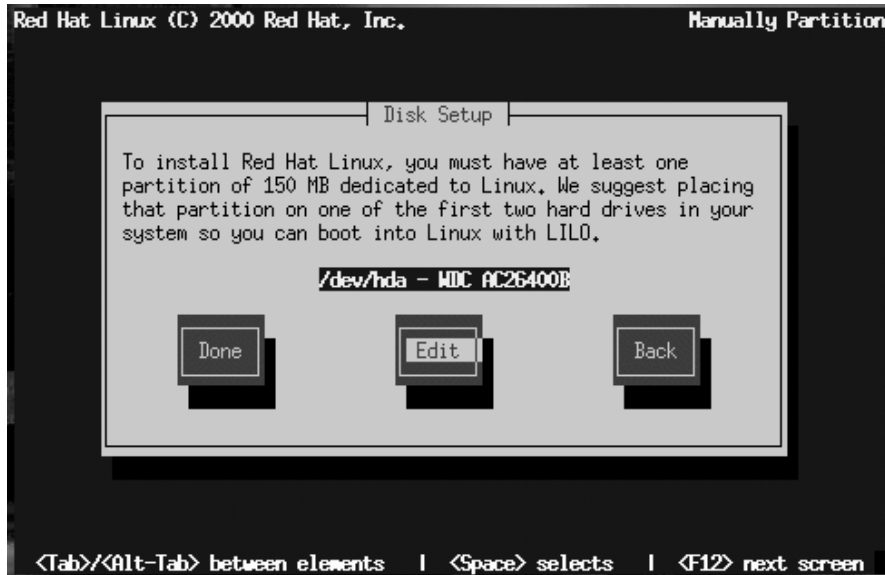
Figura 14–21 Schermata Disk Setup
