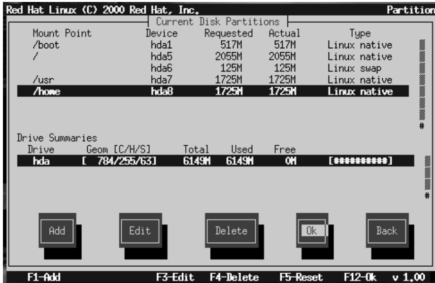
Figura 14–19 La Finestra Current Disk Partitions
