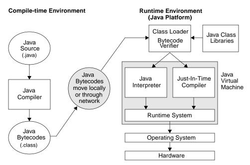
Figure 3. Source code is compiled to bytecodes, which are executed at runtime.
