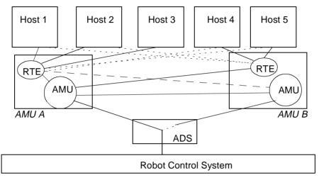
Fig. 2-2: Functional Principle Dual AMU
