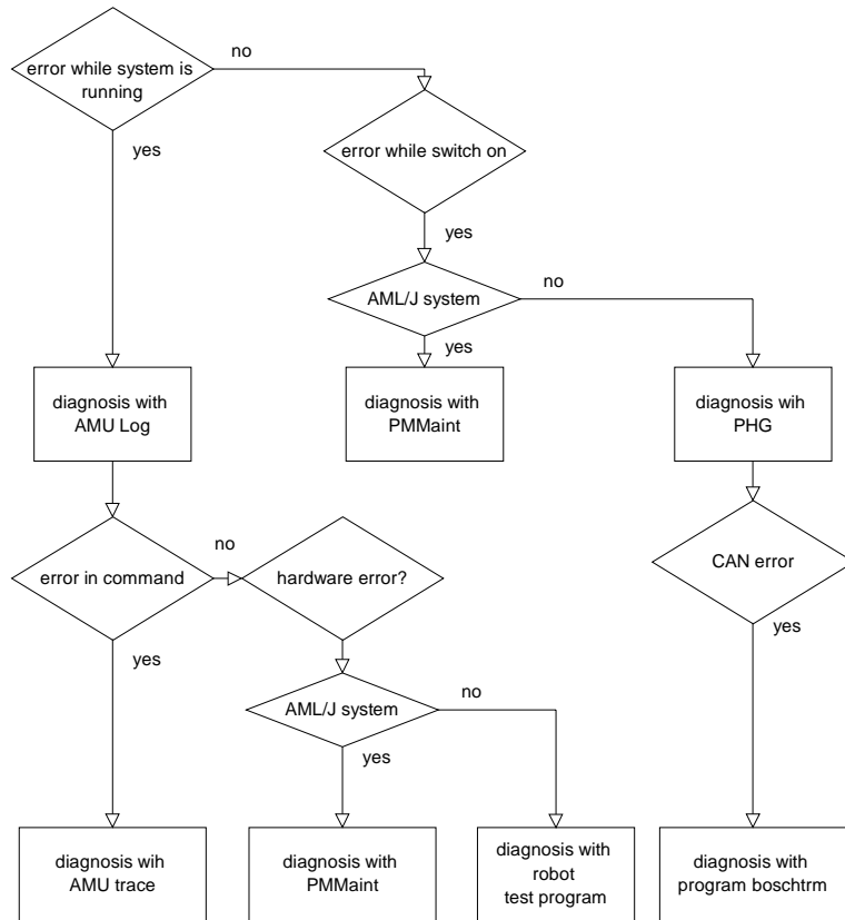
Figure 4-1: Diagnostic procedure and diagnostic tools
