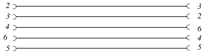
Figure 10-1: SubD 9-pole (female) to SubD 9-pole (female) (AMU<->AMU)
