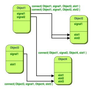
Figure 10. An abstract view of some signals and slots connections
