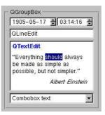
Figure 10. A QDateTimeEdit, a QLineEdit, a QTextEdit and a QComboBox laid out with a QGroupBox
