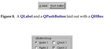
Figure 9. Two QRadioButtons and two QCheckBoxes laid out with a QButtonGroup
