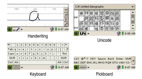
Figure 3. The standard input methods available on Qtopia
