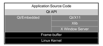
Figure 2. Qt/Embedded versus Qt/X11 on Embedded Linux
