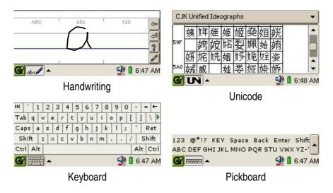
Figure 3. The standard input methods available on Qtopia
