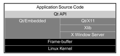
Figure 2. Qt/Embedded versus Qt/X11 on Embedded Linux
