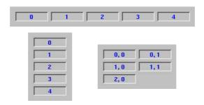
Figure 16. QHBoxLayout, QVBoxLayout and QGridLayout
