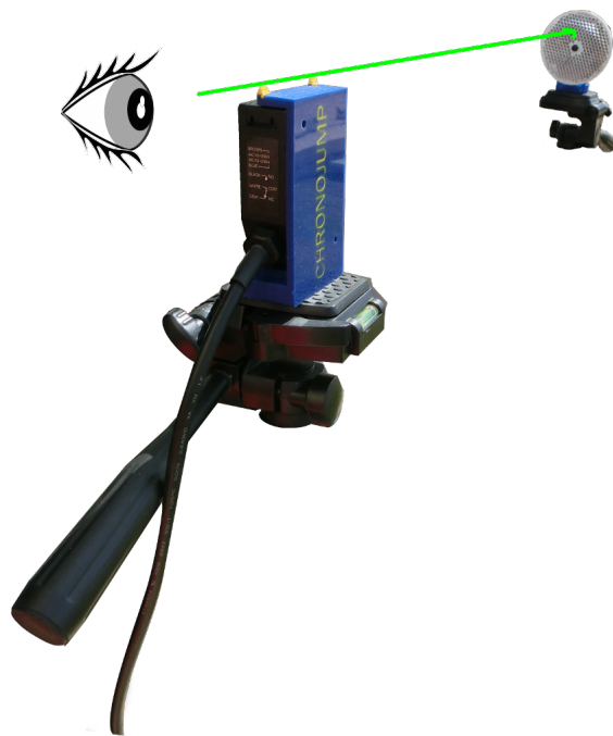
Figura 12.1: Alignment of the photocell
